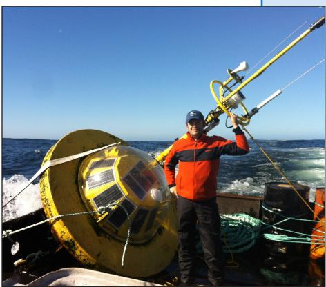
Brad Buckham offshore from Ucluelet with wave monitoring buoy from the WCWI project
