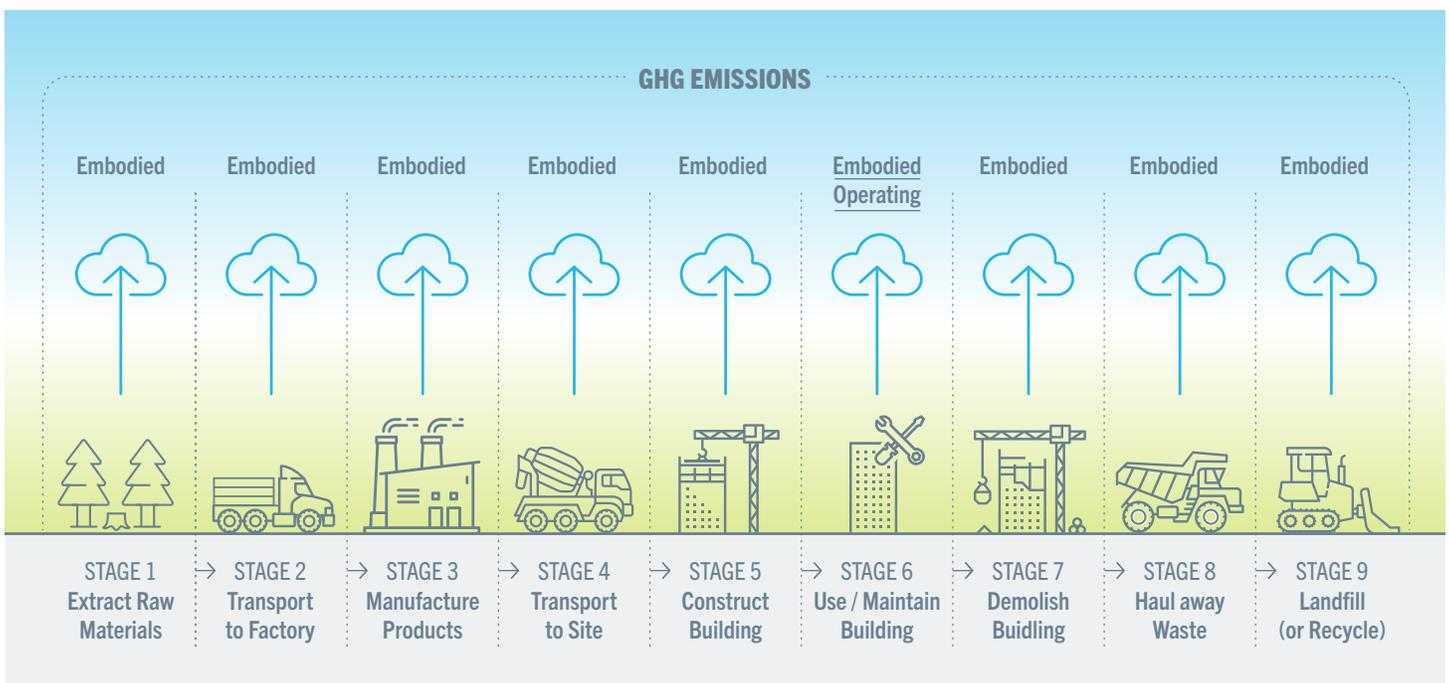
**Fig.1** Considering embodied carbon offers a more holistic perspective on the impact of construction, extending to every stage of the lifecycle rather than the narrow perspective of operations alone. [Diagram Source](#)
