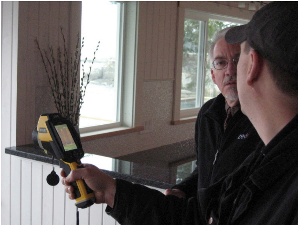
Figure 4. A thermal imaging expert conducts a real-time assessment of heat loss using a hand-held infrared camera with a homeowner. © S. Sheppard.
